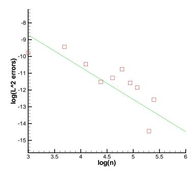
Figure 4.1: The  $L^2$  error versus the number of cells, in logarithm scale, obtained by using the first version of the central LDG methods with non-uniform meshes. The symbols (square) are the  $L^2$  errors and the solid line is the least square fit to the errors.
